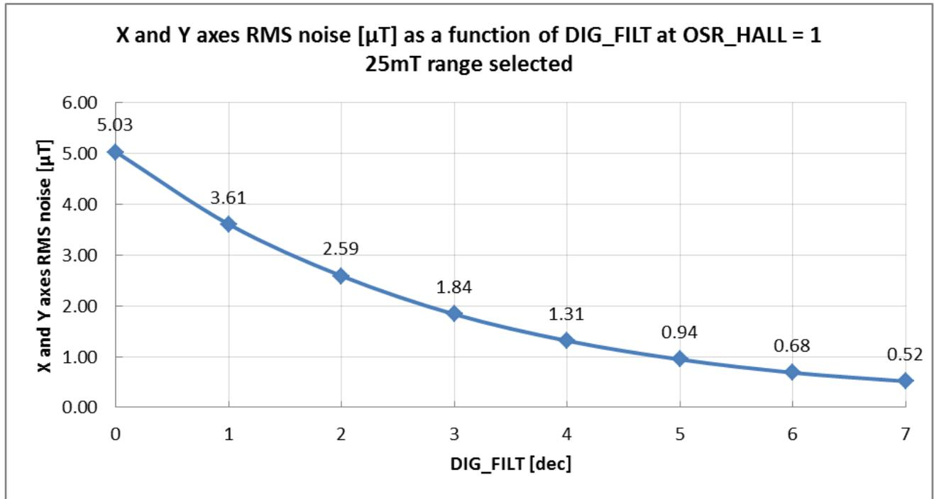
Figure 18: XY axis RMS noise (typ) without temperature compensation and 25mT range selected
