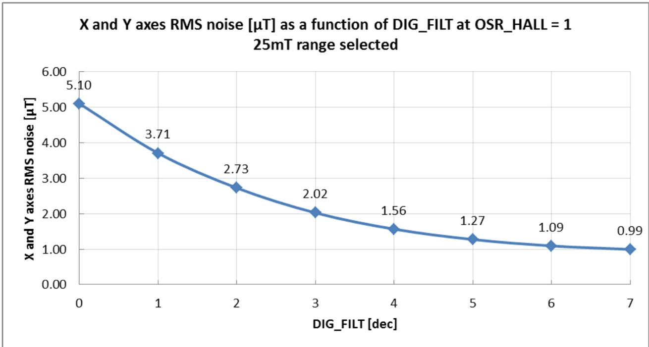
Figure 22: XY axis RMS noise (typ) with temperature compensation and 25mT range selected
