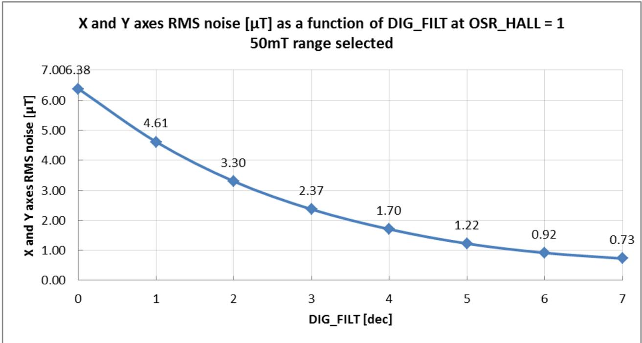
Figure 20: XY axis RMS noise (typ) without temperature compensation and 50mT range selected
